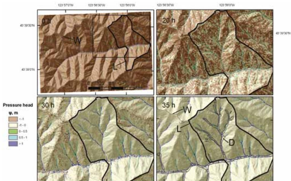
Fig. 4 - Maps showing evolution of pressure head,  $\psi$  at base of colluvium at different stages of the three rainfall periods in Fig. 3 and boundary and initial conditions depicted in Fig. 2. Rainfall after 20 h = 85 mm, after 30 h = 161 mm and after 35 h = 201 mm. Rectangle in upper left panel (0 h) indicates approximate area shown in other panels, L is logged area, D is boundaries of debris flows
