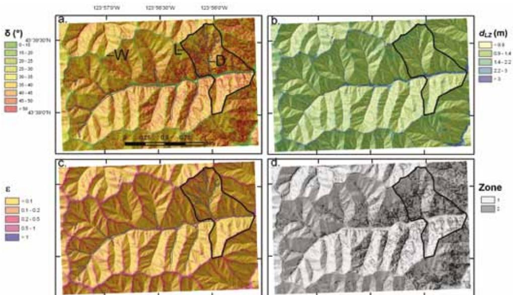
Fig. 2 - Maps showing (a) topographic slope angle,  $\delta$ ,  $W$  is watershed boundary,  $L$  is logged area,  $D$  is debris flow inventory from CoE *et alii* 2010, (b) depth to bedrock,  $d_{LZ}$  (c) distribution of ratio  $\epsilon$ , (d) property zones, 1 is colluvium and 2 is bedrock
