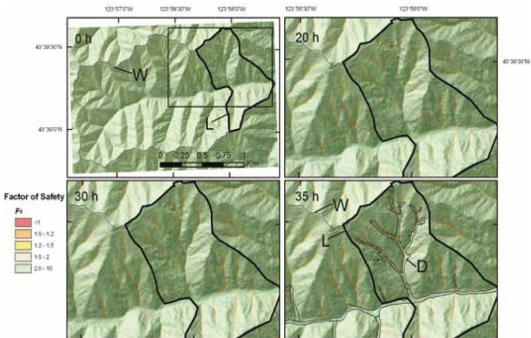
Fig. 5 - Maps showing evolution of factor of safety. Rectangle in upper left panel (0 h) indicates approximate area shown in other panels, L is logged area, D is boundaries of debris flows
