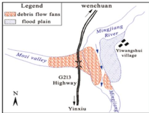
Fig. 17 - Sketch map of Mingjiang River blocked by debris flow from Mozi gully in December, 2008
